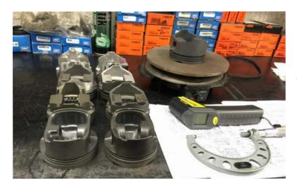
Testing the expansion rate of various past and present pistons.
