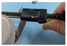
Measuring of the barrel facing, the drop off just under the oil ring groove, to be .008" or .20mm
