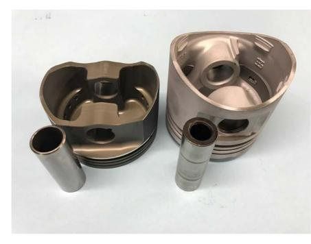
The biggest weight loses come from early model M10 and M30 engines. To the left, is a MM 2200 Rally piston that is fully machined on the backside for a maximum strength to weight ratio. The 92mm piston weighs just 315g and uses a 89g pin. The "H" beam 143mm rod used with our 2200 Rally piston and weighs 525g.
