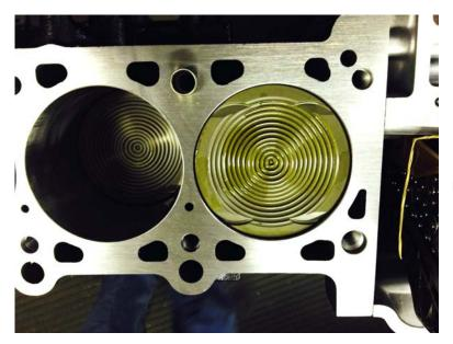
MM hard anodized Surface Turbulence (patented) piston top, used to greatly reduce detonation in our boosted Forced Induction engines.
