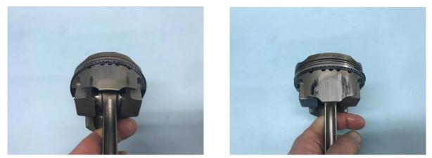
The more the skirt strut supports are placed inboard, the more prone the piston will be to piston seizure (scoring) because the skirt gets too rigid.
