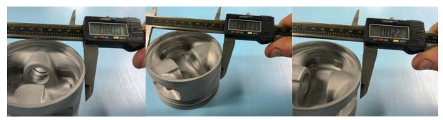
Zeroing in the caliper at the bottom of the skirt
