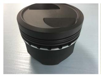
This is a current M20 hard anodize MM 3000 Sport piston with deep valve pockets. The entire piston is hard anodize except the skirt. Just under the oil ring groove you'll notice shinny aluminum thermal belt line with 5 large 3/16" oil holes, used to lubricate the textured moly coated skirt.
