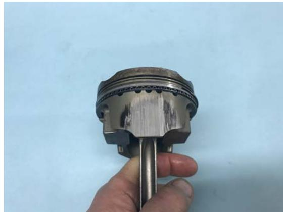
The more the skirt strut supports are placed inboard, the more prone the piston will be to piston seizure (scoring) because the skirt gets too rigid.
