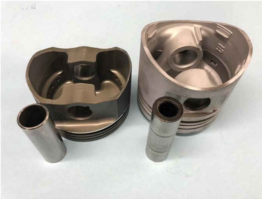
The biggest weight loses come from early model M10 and M30 engines. To the left, is a MM 2200 Rally piston that is fully machined on the backside for a maximum strength to weight ratio. The 92mm piston weighs just 315g and uses a 89g pin. The "H" beam 143mm rod used with our 2200 Rally piston and weighs 525g.
