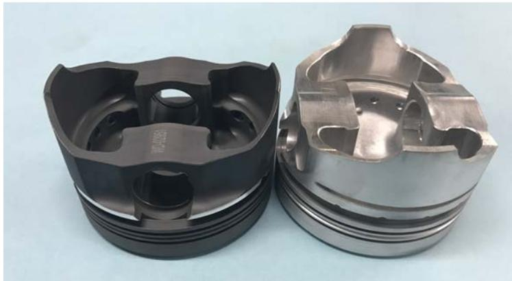
Our current piston on the left has a thinner intake (low load) skirt for greater skirt flexibility over our earlier (horizontal) slitted piston to the right.
