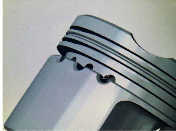
CAD designing the chamfered 3/16" oil return holes for the MM S52 3200 Sport piston.
