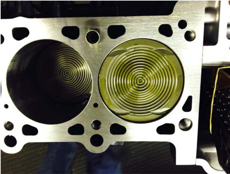
MM hard anodized Surface Turbulence (patented) piston top, used to greatly reduce detonation in our boosted Forced Induction engines.
