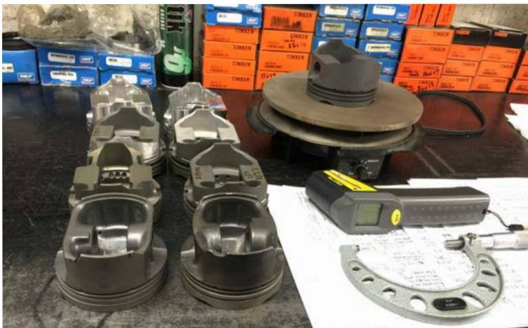
Testing the expansion rate of various past and present pistons.
