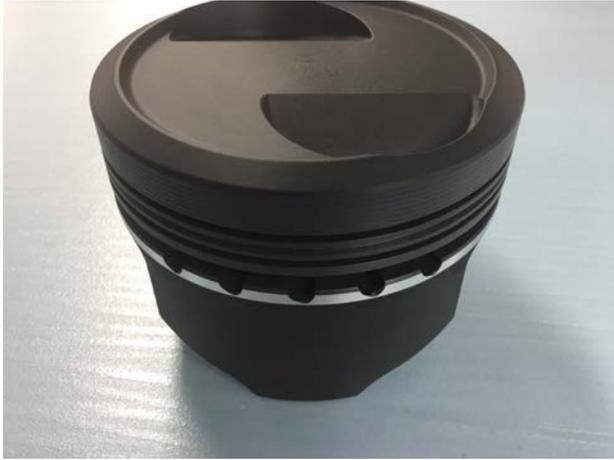
This is a current M20 hard anodize MM 3000 Sport piston with deep valve pockets. The entire piston is hard anodize except the skirt. Just under the oil ring groove you'll notice shiny aluminum thermal belt line with 5 large 3/16" oil holes, used to lubricate the textured moly coated skirt.
