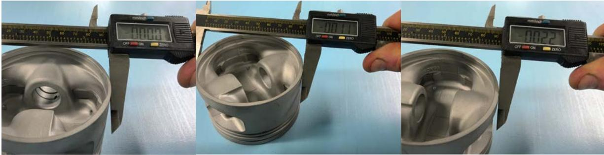
Zeroing in the caliper at the bottom of the skirt
